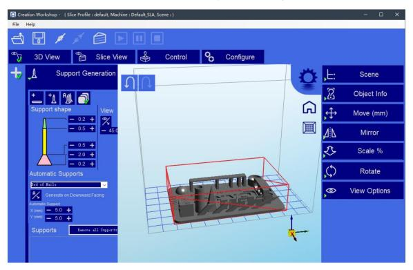
After the model has been loaded, you can add supports, as needed.
